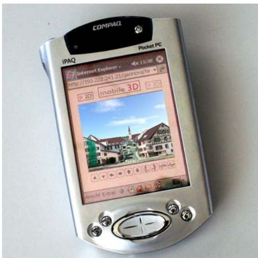
Figure 1: Demonstration 3d service «ch3d.ch» on iPaq PDA with city model of Rüslikon, Switzerland (© Osterwalder & Lehmann AG)
