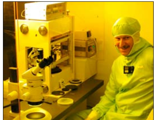
Press in cleanroom for hot embossing lithography of nano-patterns in polymer-layers
