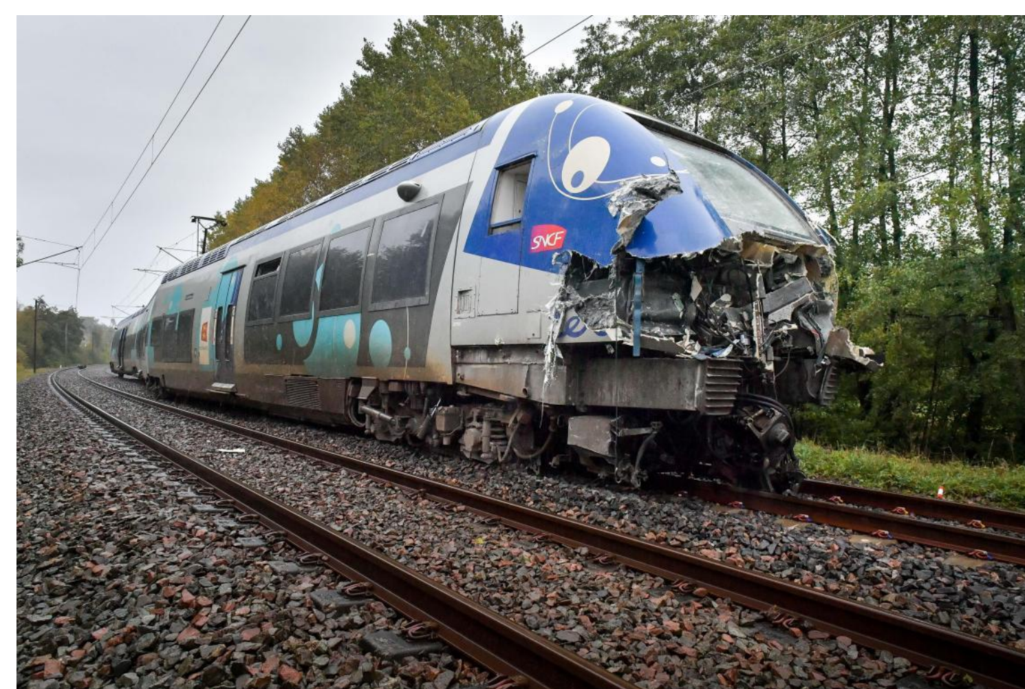
Fig. 1. Train after collision with wild boar between Cherbourg and Paris (Chasse Passion, 2020)
