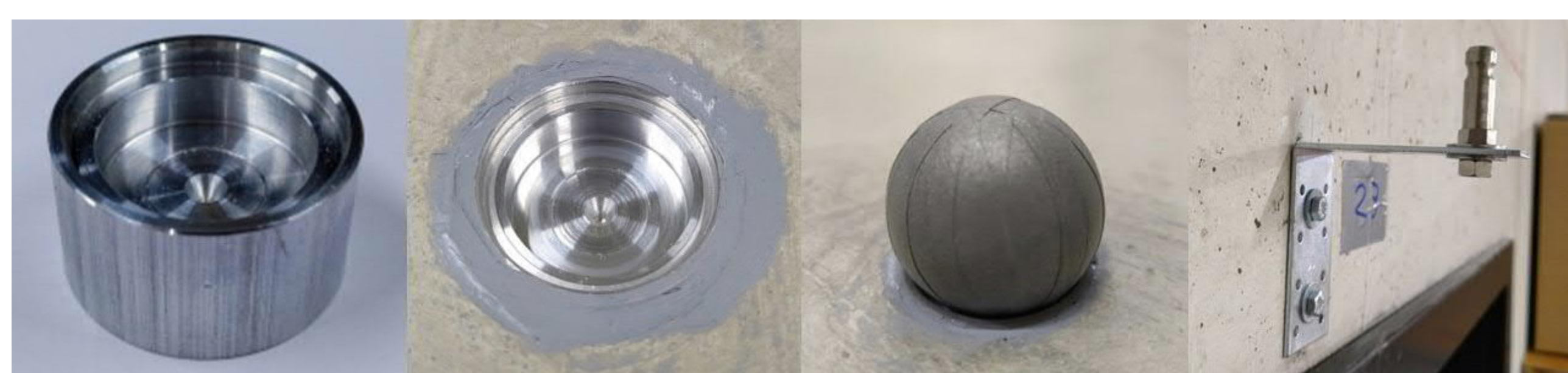
Fig. 2: The metal socket, the installed socket, a marker placed on the socket and the SBB bolt mounted to the wall with an angle.
