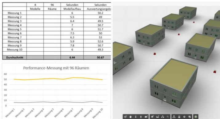
Figure 7: Test run with eight building models (96 rooms).
