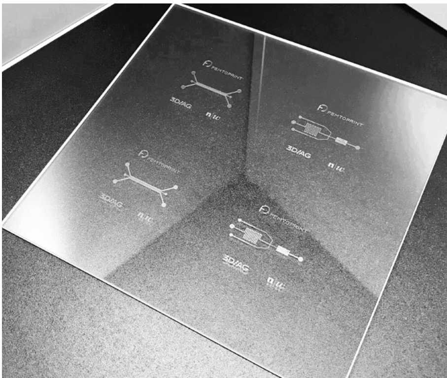
Figure 1. Example of master fabricated on 150x150x3 mm 3 fused silica substrate.
