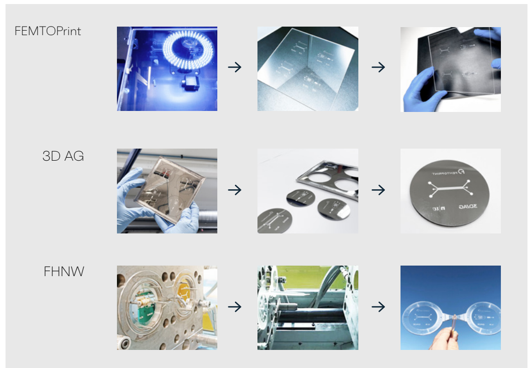
Figure 10. Case study summarising the collaborative achievements performed for this paper. Beginning in origination by FEMTOPrint (top row) through electroforming Nickel shims and tool making by 3D AG (middle row) to mass scale production by FHNW (bottom row).
