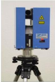
Zoller + Fröhlich Imager 5006 Multiple frequency phase-shift method Faster, lower range
