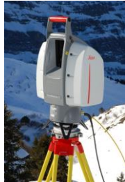
Leica Scanstation 2 Time-of-Flight method Slower, larger range
