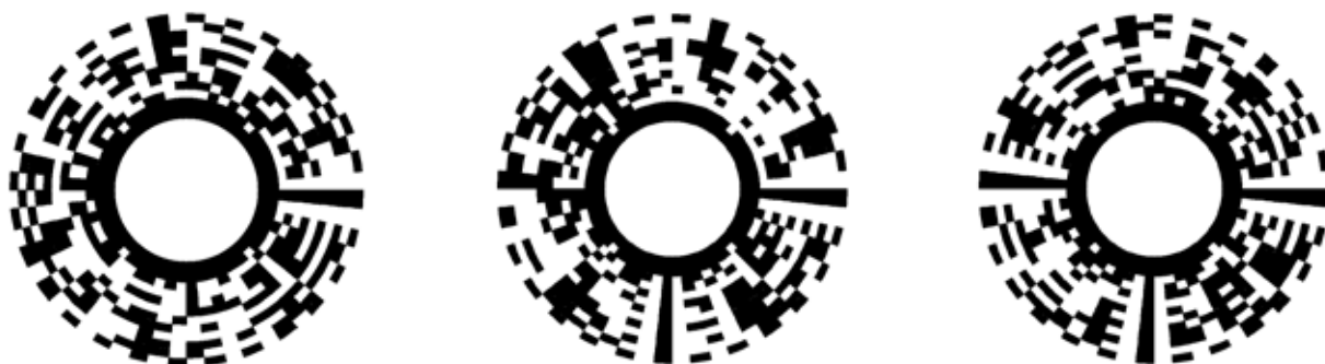
Figure 3: The three types of generic annular barcodes. Repeating start marker and radial zebra pattern increases robustness.
