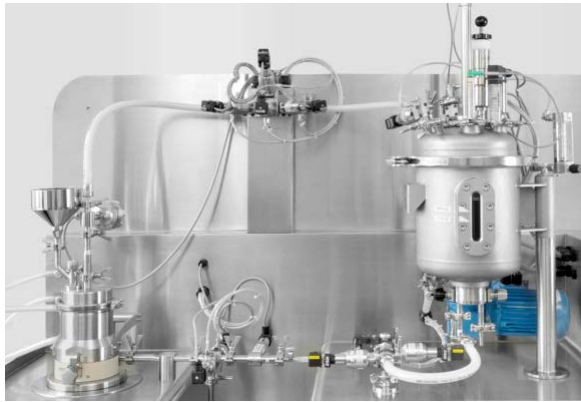
Novel type of stirred bead mill (Nanomill)
