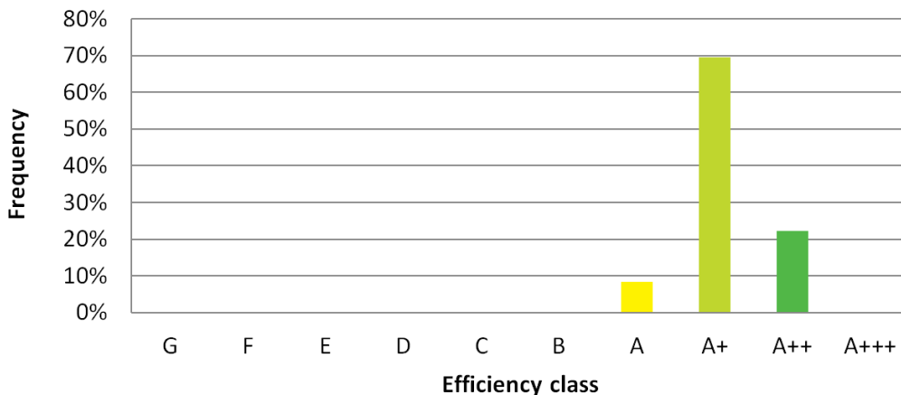
Fig. 3: Classification of actual air-to-water heat pumps on the Swiss market (Data from WPZ Bulletin [13]). Class A and higher fulfill Ecodesign requirements for low temperature (LT) application.
