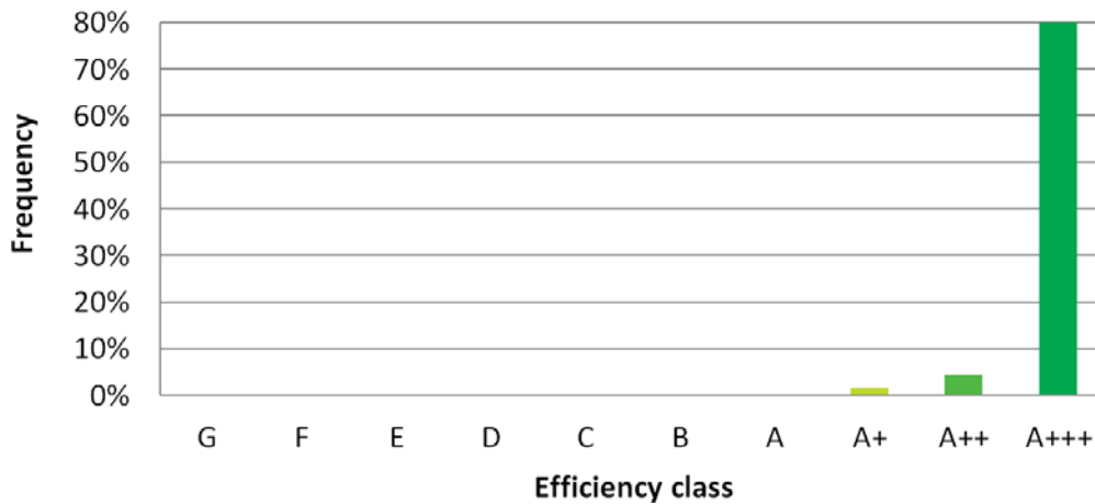
Fig. 4: Classification of actual brine-to-water heat pumps on the Swiss market (Data from WPZ Bulletin [13]). Evaluation for low temperature (LT) application. Generally, brine/water and water/water heat pumps reach high efficiency classes.
