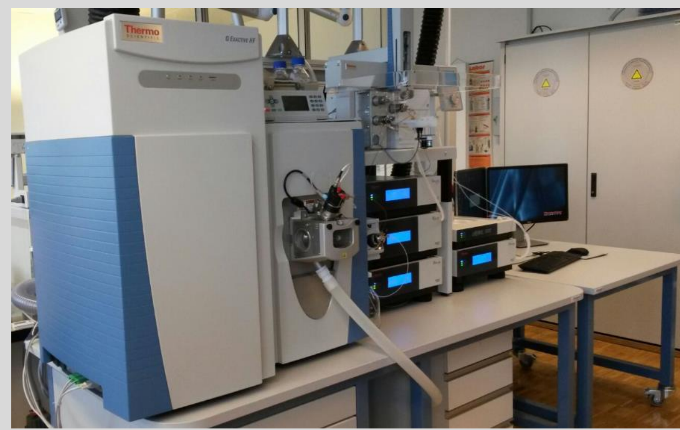
Fig.1: QExactive HF (Thermo), UPLC (Dionex) and PAL HTC sampler (Thermo)
