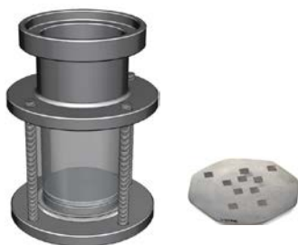
Fig. 1: Safety recipient and building platform ( \phi 65 mm) with selectively melted powder areas.
