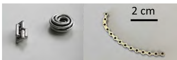
Fig. 1: Freeform magnesium AZ91 structures, produced by Selective Laser Melting.
